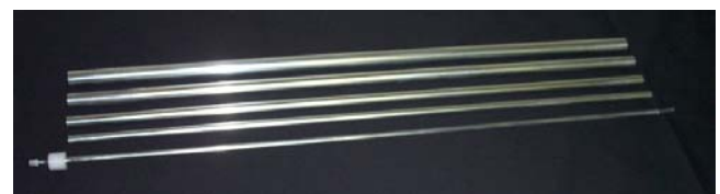
Set of aluminum tubes used in NEMA PET Sensitivity Phantom™
