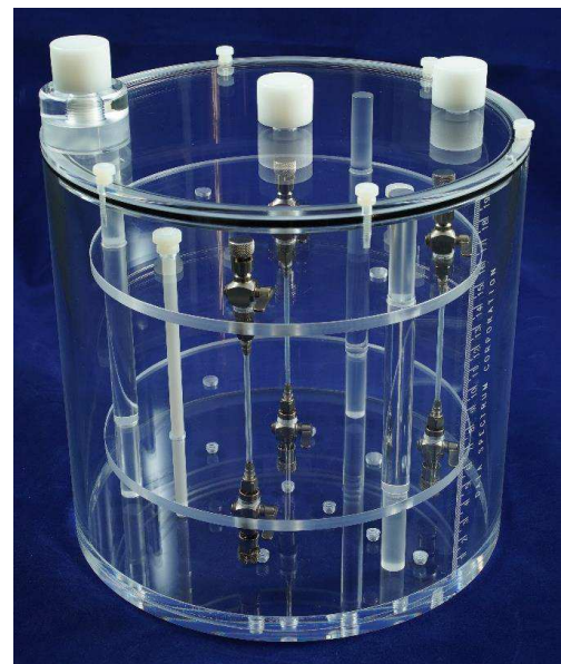
Triple Line Insert™ shown mounted inside Flangeless Circular ECT Cylinder
